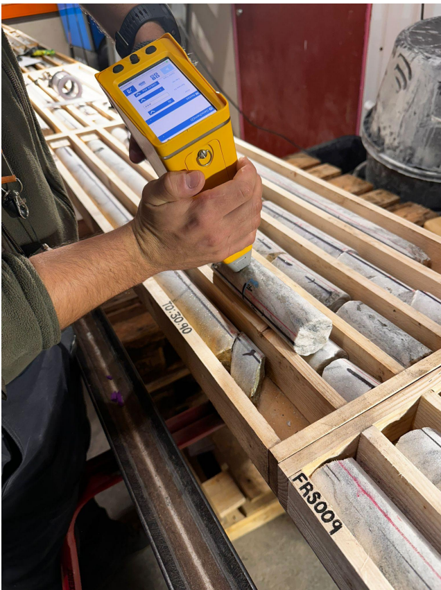
Logging of drill core at Frostmoen, the yellow device is a XRF used to identify minerals
