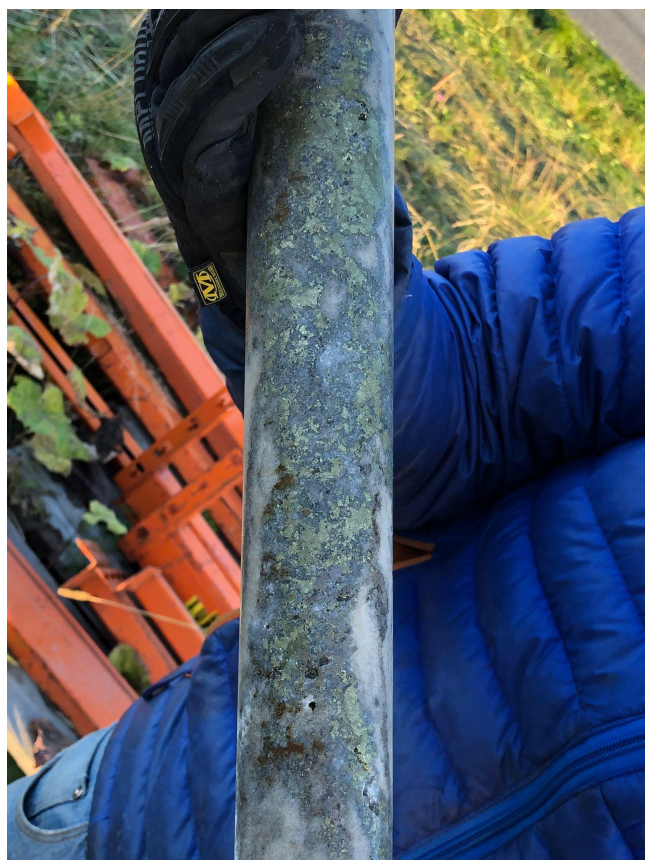
Drill core of Hole 5 with \pm 30\% of (copper) sulphide mineralization
