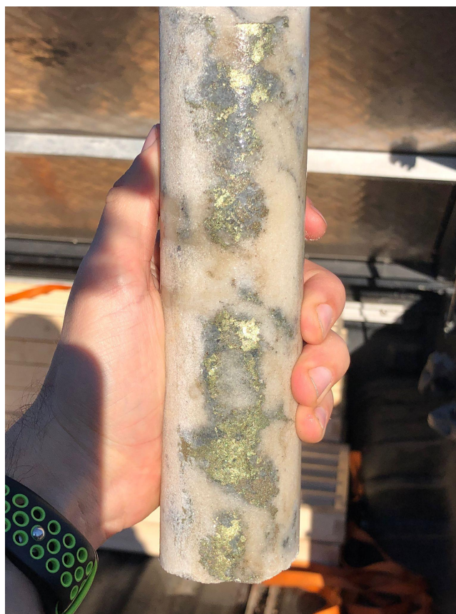
Drill core of Hole 6 with strong chalcopyrite mineralization. Chalcopyrite is a copper mineral which consists for 34.5% out of copper
