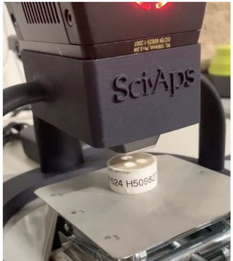
Sample about to be analyzed by the LIBS
